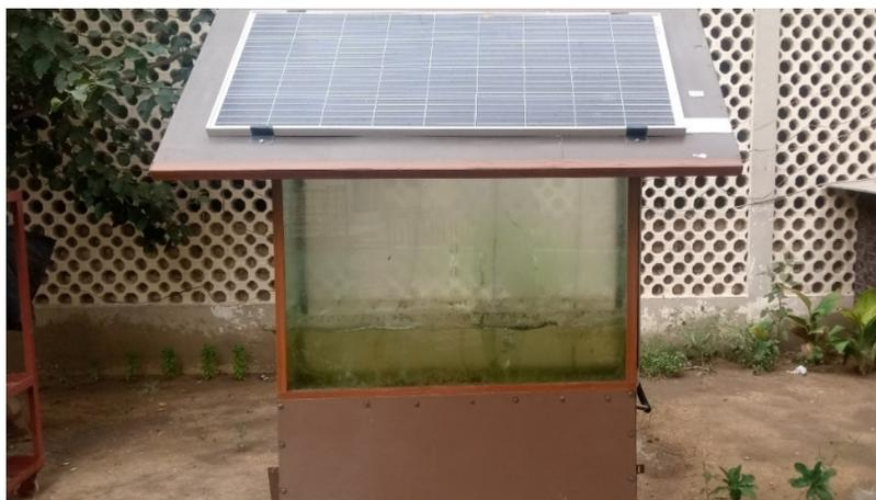
**Figure 2.** Locally designed and fabricated urban photobioreactor.
